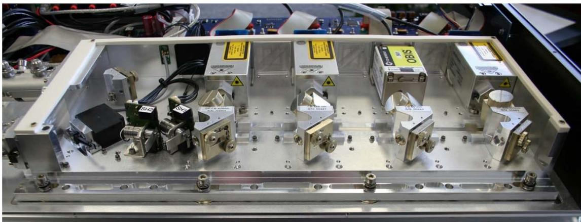
Figure 9: typical combination of three LuxX® diode lasers and one DPSS laser in the LightHUB® without frame cover
