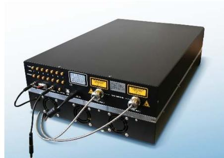
The LightHUB® ULTRA is very simple to operate, insensitive to transportation and environmental influences, to approach “hands-free operation”. Necessary control possibilities during operation are output power levels, on/off switching and modulation of the light, with all wavelengths being individually addressable via USB communication and the SMA modulation inputs at the back of the device.
